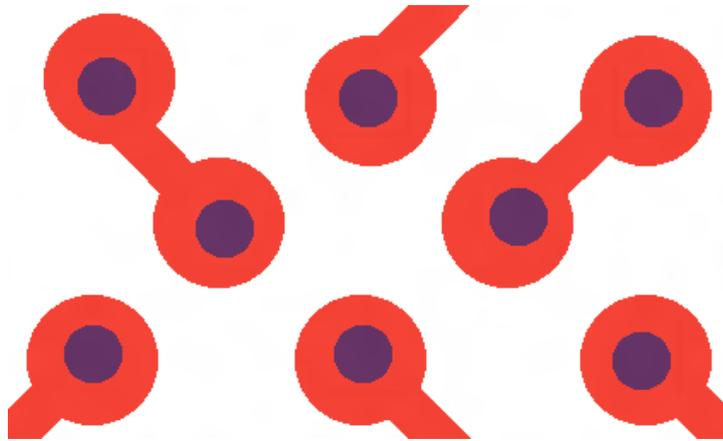
**Fig. 8 Drill and copper in different formats, not centered**
