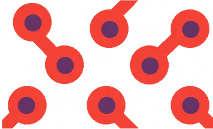
**Fig. 7 Drill and copper both in the same format, centered**
