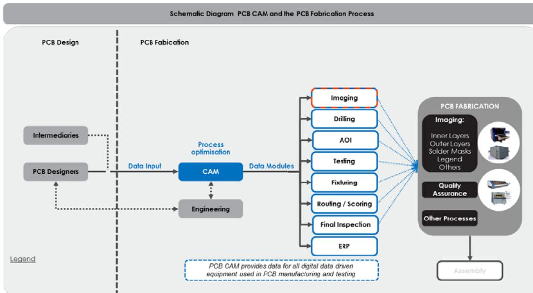
**Fig. 2 Schematic of the PCB CAM and fabrication process**
