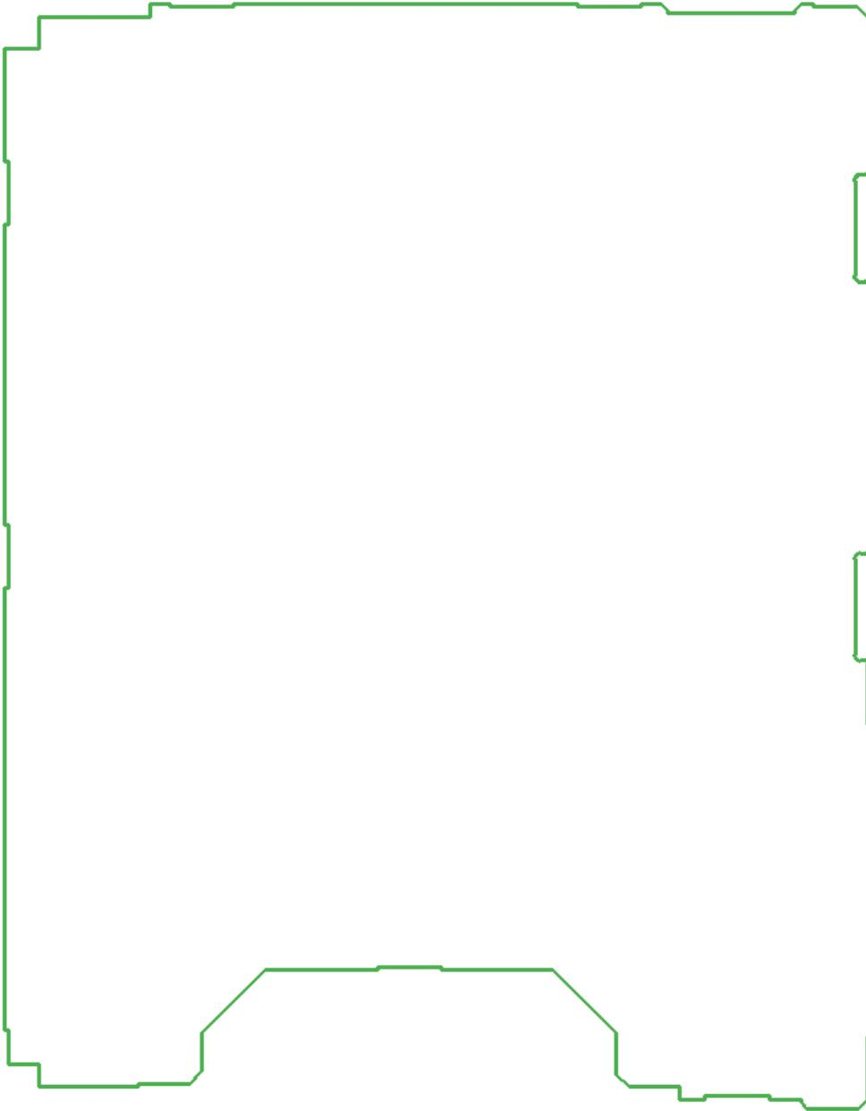
**Fig. 6 Profile stroked with a thin aperture**
