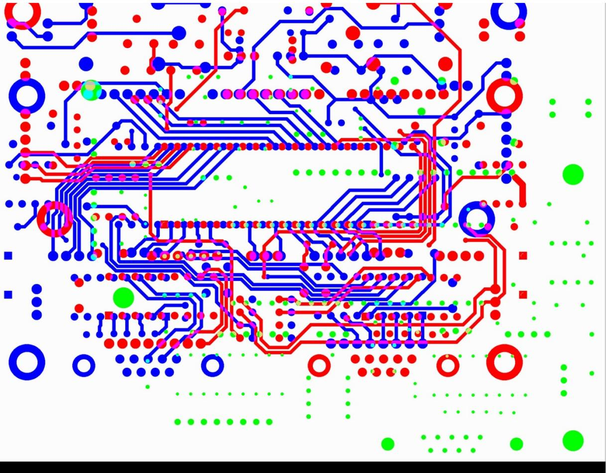
Fig. 3 Job with flipped layers and misaligned drill files
