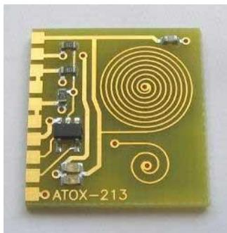
They are identified by the .AperFunction attribute value 'EtchedComponent' attached to the aperture used to create them. See <Cross-reference>.
