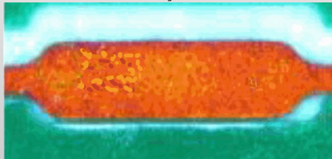
SMD after etching without horns
