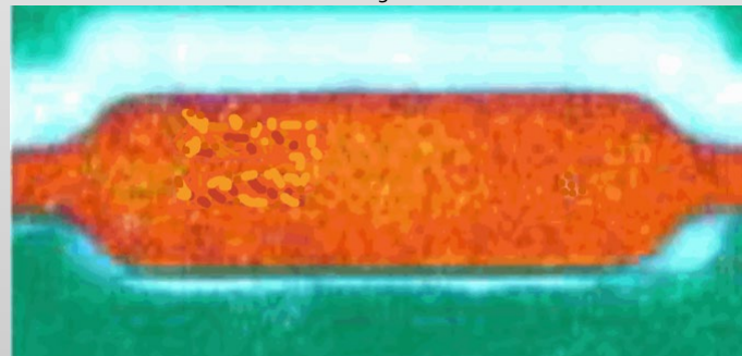
SMD after etching without horns
