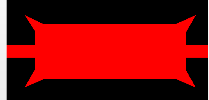
SMD with horns before etching
