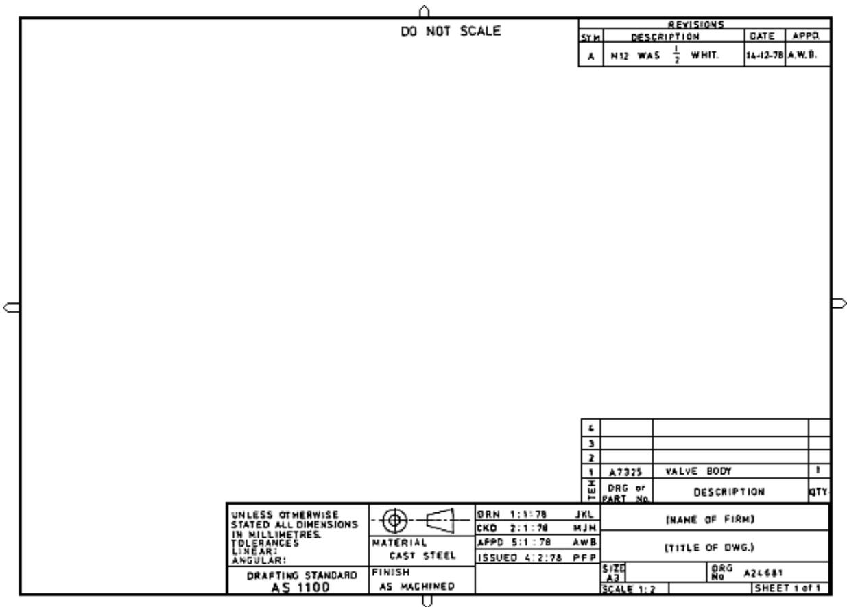
Fig. 11 A typical frame for a technical drawing
