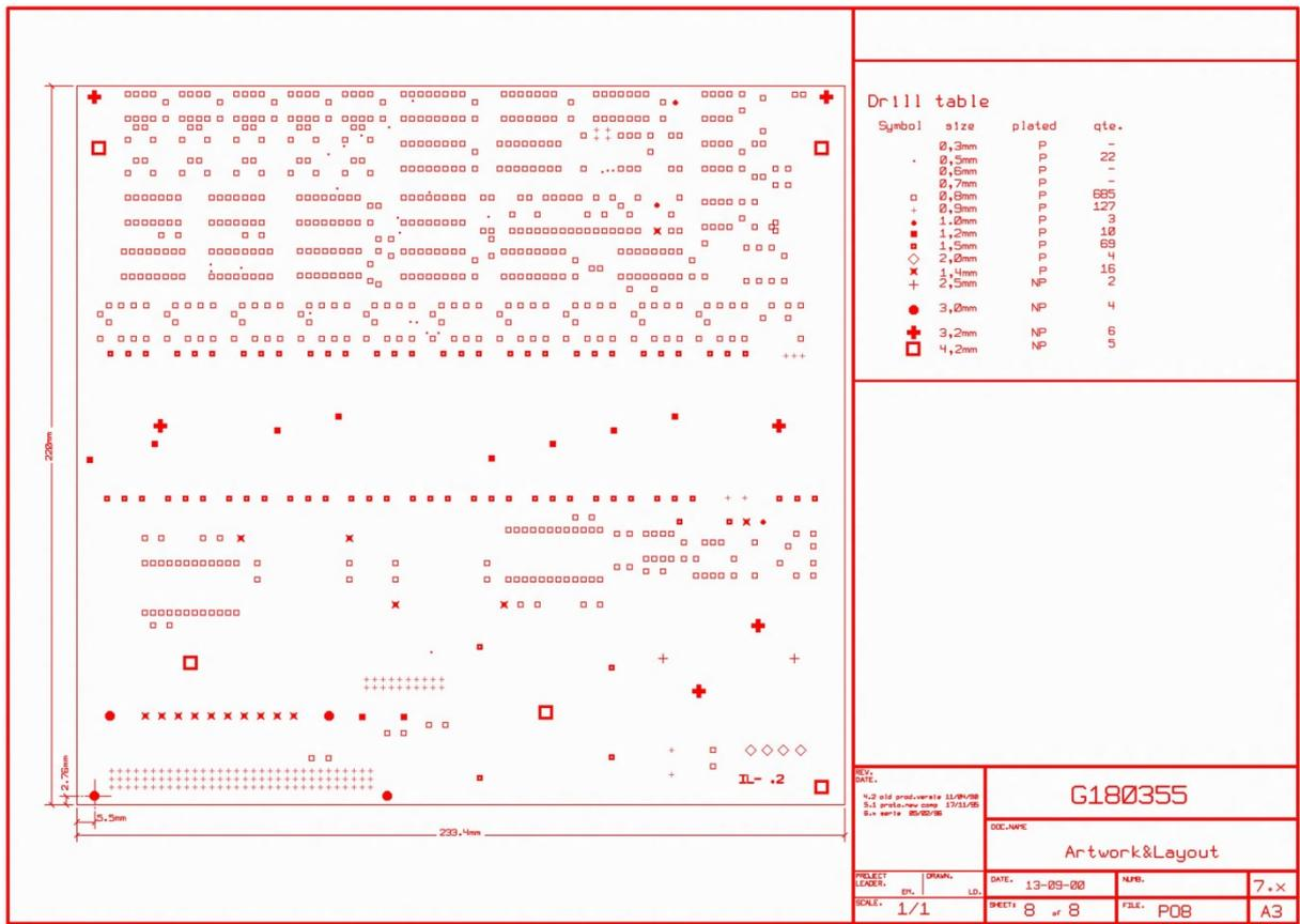
**Fig. 10 A drill map. Useful maybe, but not a substitute for drill data**
