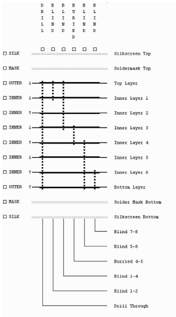
**Fig.9 The layer structure**
