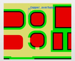
**Ring mask to pad for SMDefined pads** Overlapping of Soldermask on copper at Soldermask defined pads.
