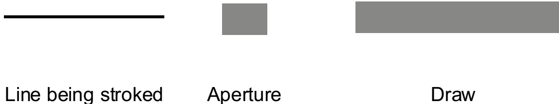
53. Creating a draw: the aperture is aligned with line
