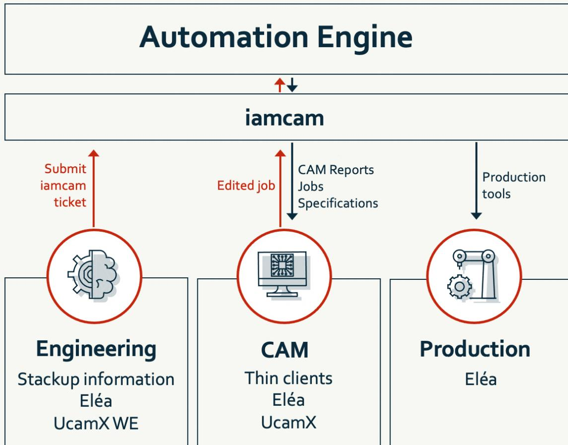
cam ticket defined specific requirements such as minimum annular rings and clearances, depending on IPC classification, copper weights, layer count, etc. And if all the requirements were not quite reached but close, it listed the type and scale of edits that the system was approved to make without having to refer the job back to the customer.
