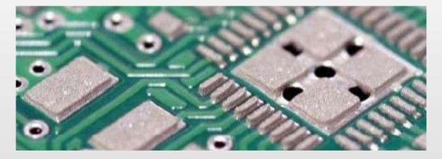
amounts of solder paste must be calculated and the stencil must be shaped accordingly.
