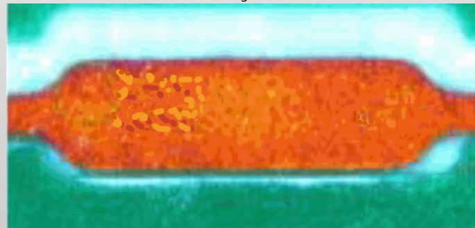
SMD after etching without horns
